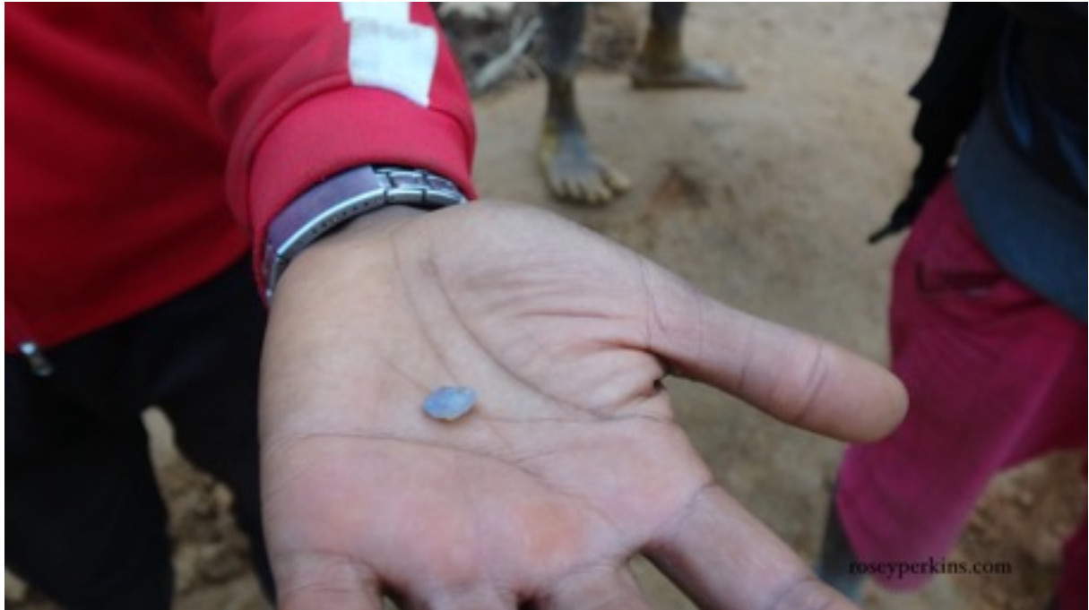
Figure 18: Milky blue sapphire called "geuda" by Sri Lankan traders. These stones are heat treated to become (hopefully) transparent and blue Photo: Rosey Perkins.
